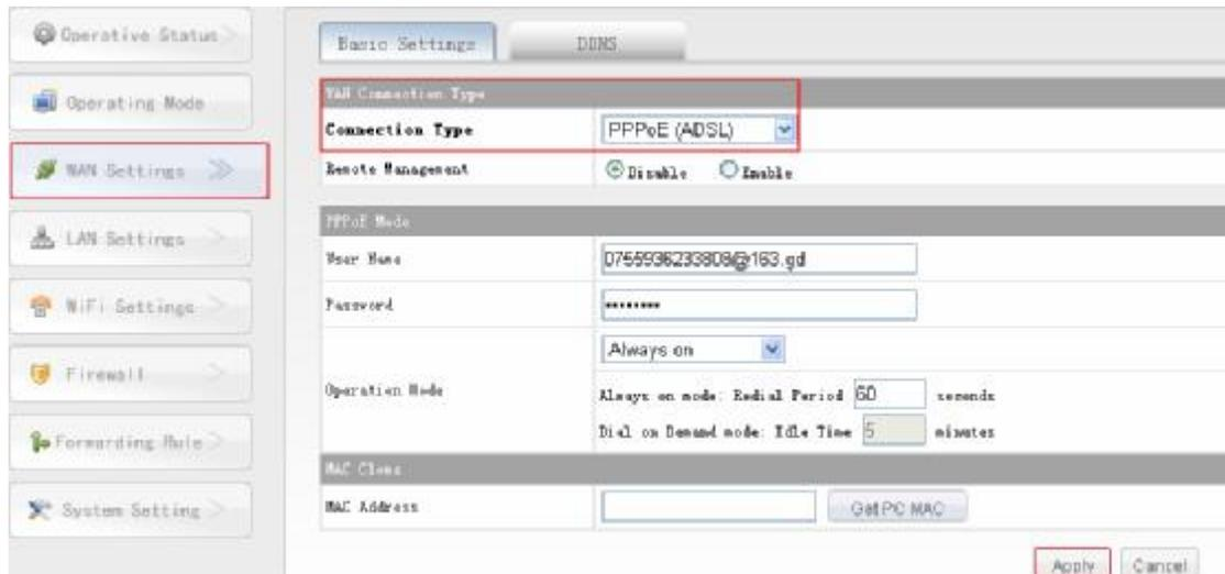
The screenshot shows the WAN Settings page with the Basic Settings tab selected. The Connection Type is set to PPPoE (ADSL). The Username is 0755936233808@163.gd and the Password is masked with asterisks. The Operation Mode is set to Always on. The MAC Address field is empty, with a Get PC MAC button next to it.
