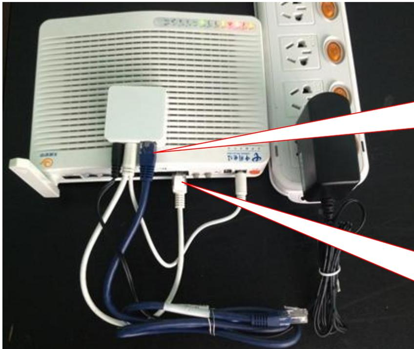
RJ45 ethernet port of VAR11N, can be used as LAN and to connect computer or LAN extension
