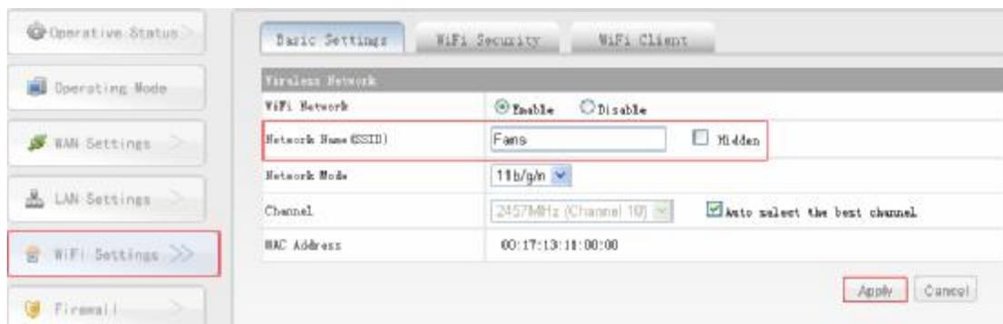
The screenshot shows the WiFi Settings page with the Basic Settings tab selected. The WiFi Network is enabled. The Network Name (SSID) is set to Fans. The Network Mode is 11b/g/n. The Channel is 2457MHz (Channel 10). The MAC Address is 00:17:13:11:00:00.
